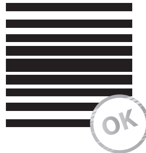
Fig. 2 PASS The stripes on the test sheet are uniformly black or anthracit grey. The colour change is homogeneous.
